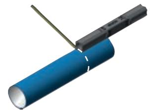
The mark will be done with any common stencil and should appear close to the nut end in order to check the correct depth of the pipe insertion into the fitting.
