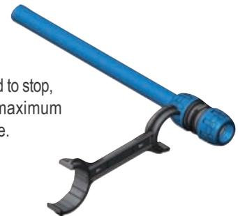
**7** A correct fitting tightening will bring the ring nut base to stop around the middle of the tightening indicator. The nut brake will act as anti-screwing in case of light vibrations.
