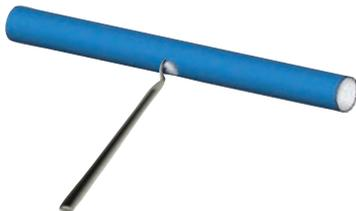
**5** Remove the branch and clean the hole with the help of the special deburring tool
