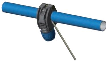
**2** Mark the chosen position near the reference notches
