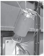
Air cannon is used to give support to free-flow of material in bunkers, hoppers, silos, etc. The volume of reservoir of air cannon is intensely expanded into the area with blocked material. This shot will release the material, which will flow by standard way.
