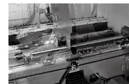
Coolant Through Ball Screw 3 axes feedrate 48M / 60M (Optional)
